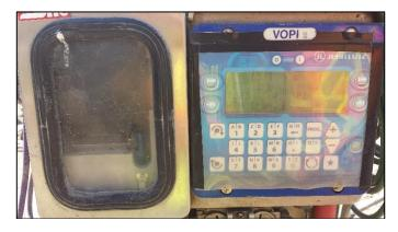
The grouting operation was monitored by an Automatic parameters register from Jean LUTZ VOPI2, controlling the flow rate, the pressure and the intake of Sodium Silicate mix in each valve.
