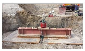
Before the start of the production soil anchors and to confirm the design solution a campaign of verification test take place in three sacrificial soil anchors tested at 200% the Design Load.
